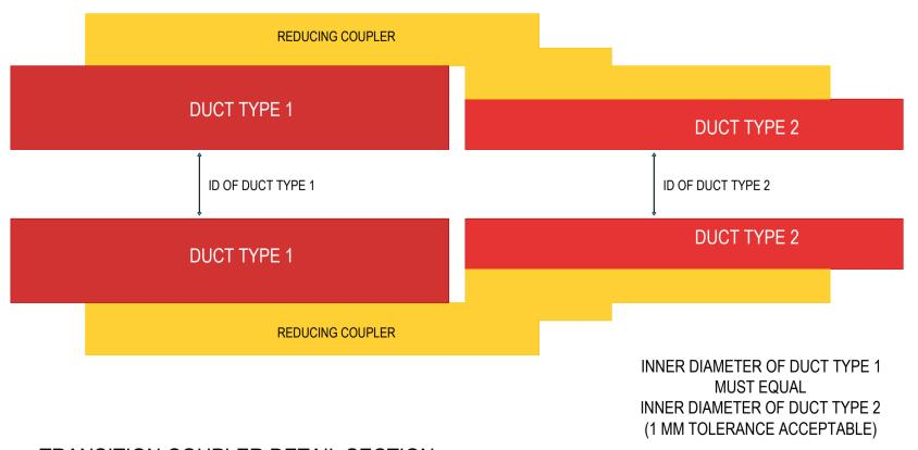
TRANSITION COUPLER DETAIL SECTION SCALE NTS
